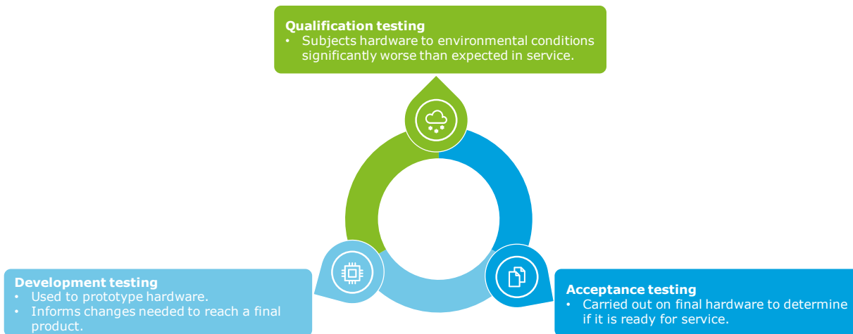
Figure 4.1 Aerospace hardware testing stages
